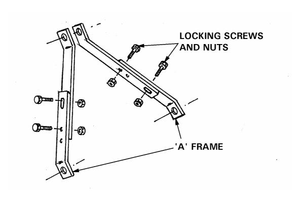
The 4 bolts (2 each side) of 'A' frame, once fitted to bars at chosen length setting position, MUST be left slack at this stage of the assembly.
