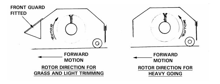
IMPORTANT For cutting upwards, the cutting head front guard must be FITTED.
