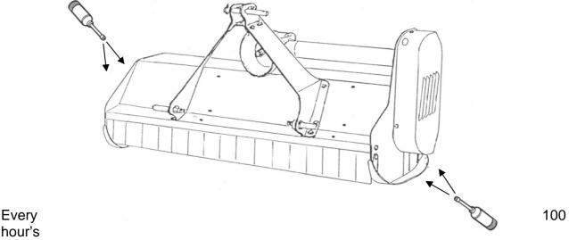
operation grease the moving parts of the PTO shaft, extracting the two parts of the shaft.
