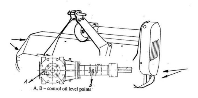
This operation must be always carried out at the end of each working day. This facilitates the removal of mud or other material form the rotating parts (bearing, pins etc.) in order to avoid rust and possible seizure.
