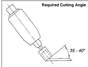
A high speed hand grinder should be used, with ideally, a pot shaped pencil grinder of approximately 1" (25mm) diameter by 1 3/8" (35mm) long. Grinding is carried out with the end face of the grinder moving from the base of the knife section up to the points.
