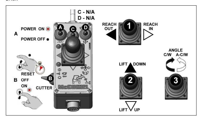
Before commencing work it is advisable to find an unobstructed level site and operate the machine through its entire range of movements to familiarise yourself with the controls and the machines response to them. This is a wise precaution for all operators and a must for the inexperienced.
