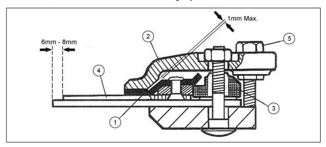
When adjusted correctly the knife sections (4) lie flush between the fingers and the underside of the knife holder (1) with the fingers projecting 6mm to 8mm in front of the knife tips. In addition there must be a maximum clearance of 1mm between the sloping faces of the knife holder (1) and the guide plate (2). This allows clearance for the knife to move freely and can be checked by placing a 5/8" dia bar into the con rod socket in the knife heel and operating by hand.
