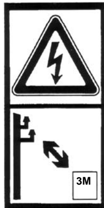
AVOID OVERHEAD CABLES DANGER OF ELECTRIC SHOCK
